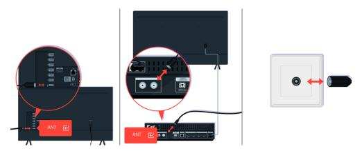
Check the antenna and input cable connections.
