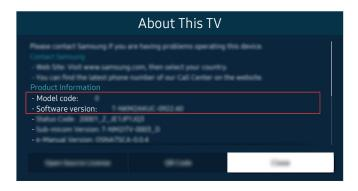
After your TV has been reset, select  $\textcircled{a} > \equiv \text{Menu} > \textcircled{8} \text{ Settings} > \text{Support} > \text{About This TV} \text{ and check the new firmware version.}$
