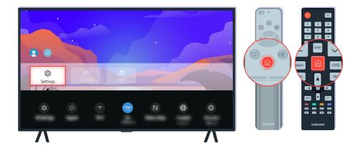
After your TV has been reset, select  $\textcircled{a} > \equiv \text{Menu} > \textcircled{8} \text{ Settings} > \text{Support} > \text{About This TV}$  and check the new firmware version. Iry Now
